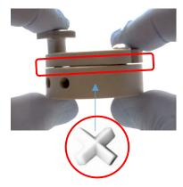
3. Each end of pipe has a nut and ferrule (note the direction of the ferrule – cone into the fitting!). Pipe fittings (and blanking nuts) are installed "finger-tight".
